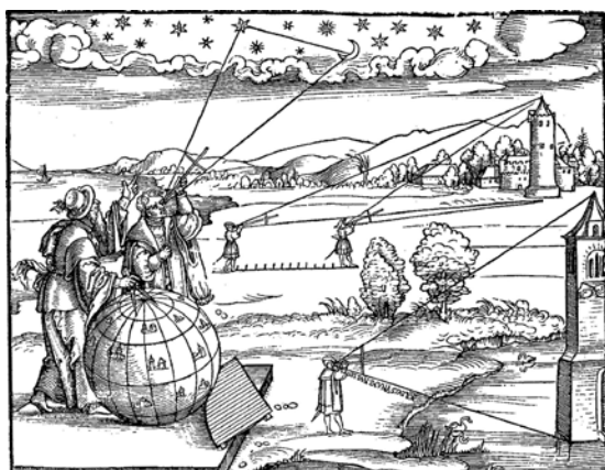
Fig. 17. Using a cross-staff to find longitude by lunar distance from stars. Woodcut in J. Werner and P. Apianus, Introductio geographica Petri Apiani in Doctissimas Vernerii annotationes , Ingolstadt, 1533. Illustrated by J. A. Bennet, The Divided Circle – A History of Instruments for Astronomy, Navigation and Surveying , 1987, p. 56
